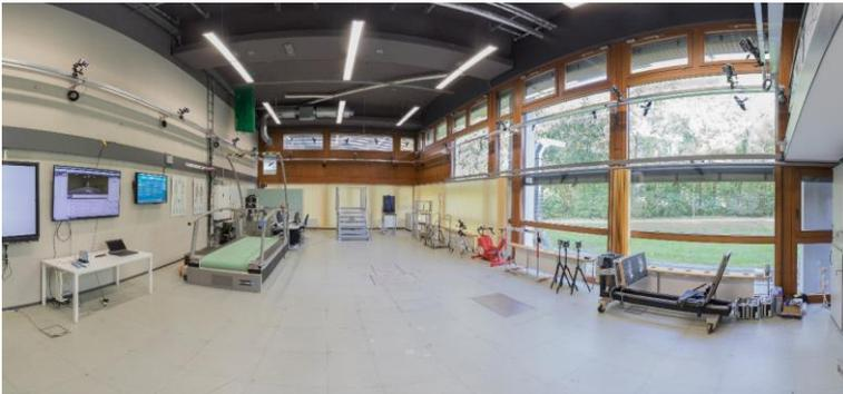
**Measuring systems:** Motion capture, high speed video, force plates, pressure measuring systems, instrumented stairs, strength diagnostics systems, EMG, EEG, Posturomed, stability platform, fall simulation tool, treadmill, SRM ergometer, mobile sensors (e.g. IMUs)...
